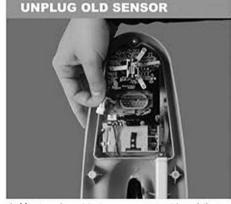
4. Unplug the old temperature and humiditye sensor by grasping the base of its whitee plug and gently removing it.e
