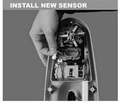
6. Slide the new temperature and humiditye sensor into place. Holding the base of itse white plug, gently plug it into the connector, e
